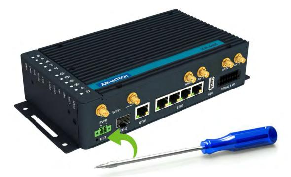
Figure 23: Resetting the Router
