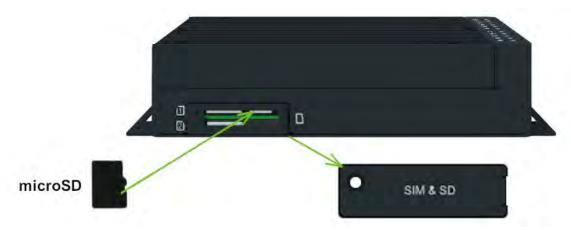
Figure 22: MicroSD Card Insertion
