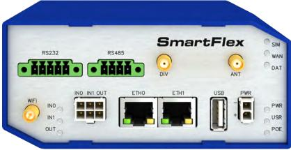
Figure 26: SmartFlex front panel
