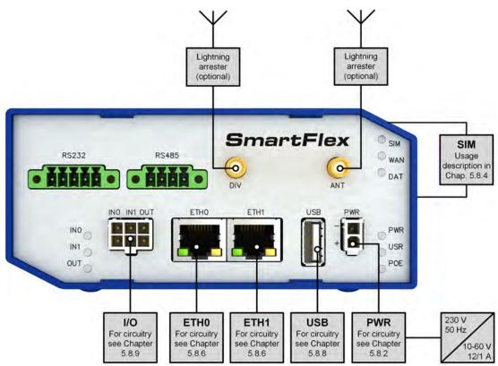
Figure 51: Router connection
