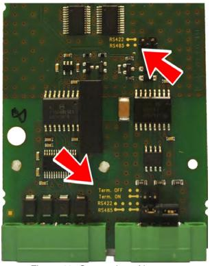
Figure 46: Connection of jumpers
