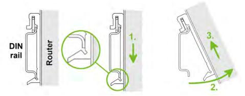
Figure 25: Removal from the DIN rail
