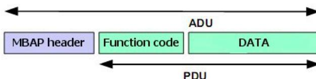
Figure 3: Modbus message on TCP/IP
